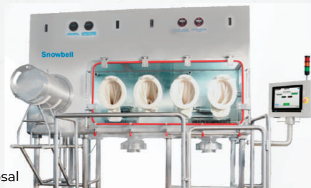
Sampling and Dispensing Isolator
